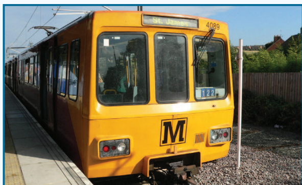
LRT – Light Rail Transit. Lighter Electric Trains better suited to operating high frequency services with close stop spacings than EMUs. The best example in the UK is perhaps the Newcastle Metro. Could be considered on the core Valley lines network instead of EMUs.
