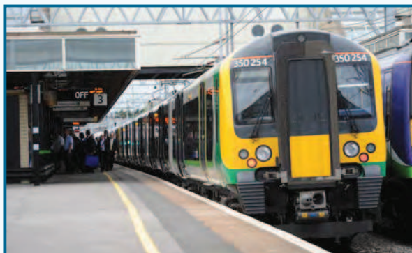
EMU – Electric Multiple Unit. Standard ‘heavy rail’ Electric Commuter Trains in widespread use across the UK and likely to be rolled out on some/all of the valley lines network following electrification by 2020.
