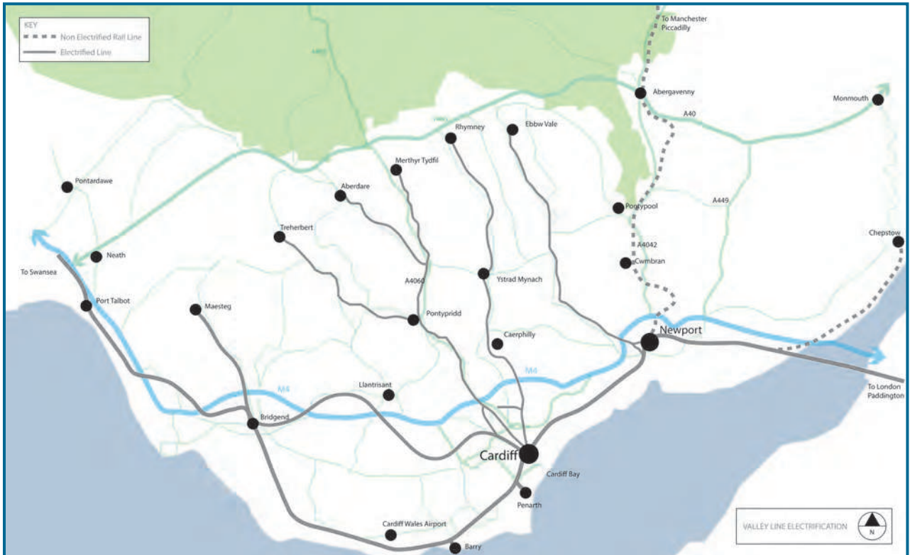
Figure 35: Scope of Valley Lines Electrification
